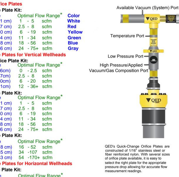
\* For best practice and most efficient operation, use the next smaller orifice plate when the pressure differential is less than 0.5 inches of water column; Use the next larger orifice plate when the pressure differential is greater than 5 inches of water column.
