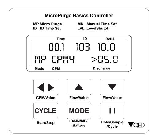
In this mode the CPM and UP, DOWN keys function differently. The CPM key becomes a key used to scroll between the one's and the ten's digits of the ID. The UP and DOWN keys are used to change the ID number (the MP50 has IDs that range from 1-165) up or down in value. Sampling in ID mode is the same as explained, above, for MP mode.
