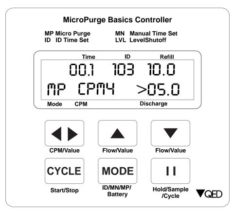
**Using CPM** The MP50 introduces a revolutionary, simpler way to control bladder pump flow rate and achieve the low-flow method used by experts. Up/down arrow keys are used to adjust pump flow even at very low rates, with excellent control and repeatability.
