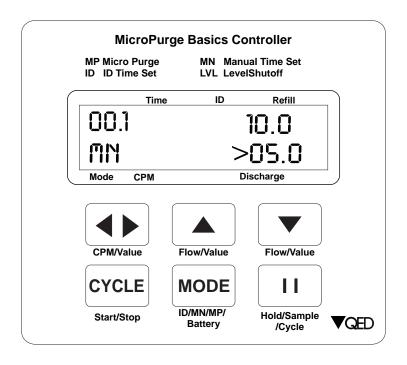
In User Set mode the CPM and UP, DOWN keys function differently than MP mode. The CPM key becomes a key used to select the digits of the refill and discharge time settings found at the rightmost positions on the display. The UP and DOWN keys are used to adjust the digit value up or down. By selecting and adjusting digits up and down a user can quickly set any time from 00.1 seconds to 99.9 seconds. Sampling in User Set mode is the same as explained, above, for MP mode.
