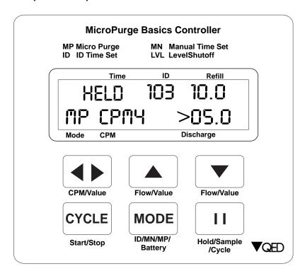
**Warning:** in the HELD SAMPLE state the pump, tubing and hoses are all under pressure. **DO NOT** attempt to disconnect or disassemble any part of the system when it is under pressure. The system is under pressure if the pressure gauge shows a value greater than 0 and the RED Discharge Cycle Indicator is showing.
