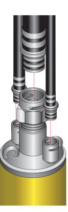
5. Push retaining clips into their mating retaining slots. Push clip into slot until it "clicks" into its locked position.
