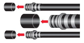
**IMPORTANT NOTE:** The smallest fitting is the air supply. This fitting needs to be inserted into the pump hole marked "I". The next larger fitting is the air exhaust fitting. This fitting needs to be inserted into the pump hole marked "E". If these two fittings are not installed into the correct holes the pump will not operate. It is easiest to insert the discharge line first then insert the pin, then either the air or exhaust and pin.
