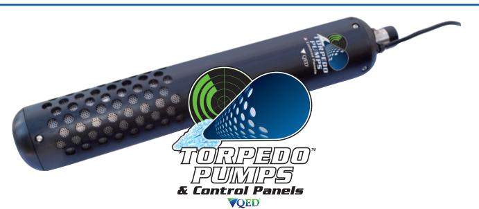
QED Torpedo<sup>TM</sup> electric submersible pumps are made of stainless steel and fitted with teflon seals and bearings to handle the rigors of contaminated groundwater pumping and continuous operation in landfill/remediation applications. Built to deliver optimum efficiency periods of high demand, all electric pumps provide low, long-term
