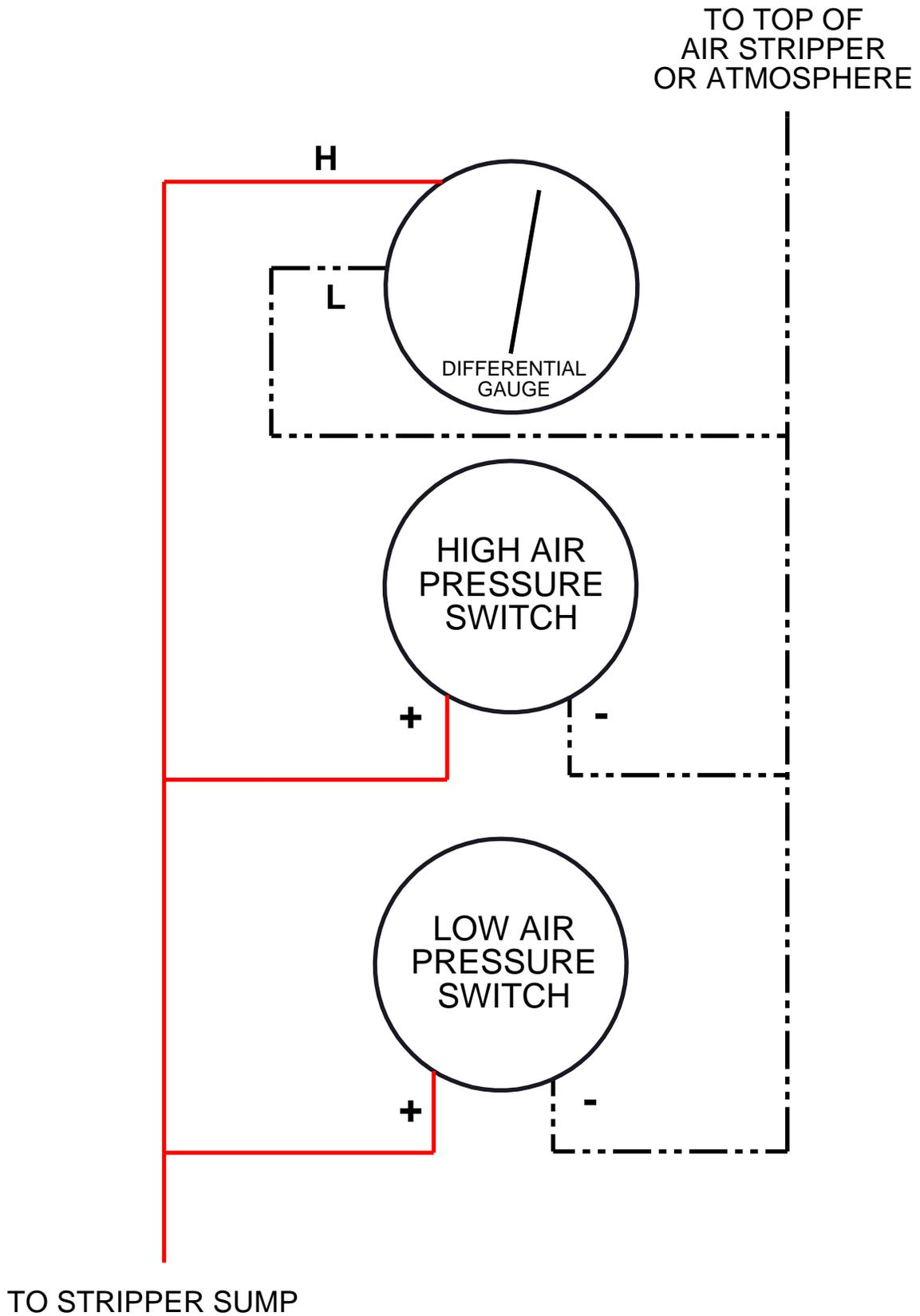
AIR STRIPPER GAUGE AND PRESSURE SWITCH CONNECTION DIAGRAM (Optional)
