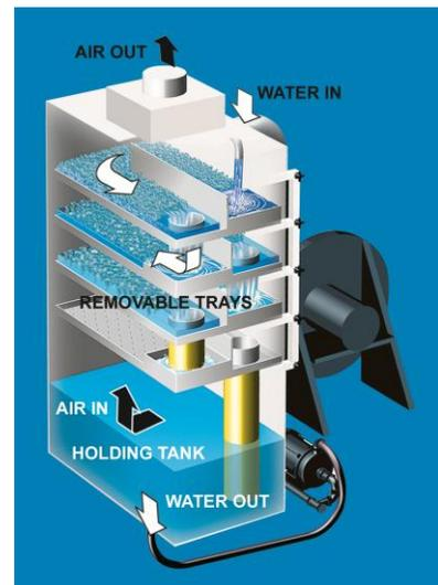
The counter current flow of a tray air stripper.
