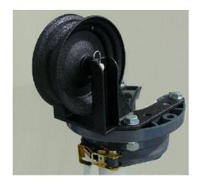
The QED Pump Puller was designed to facilitate the removal of pumps from deep wells. The pump tubing is laid over the rotating wheel (pulley), allowing the tubing to be pulled horizontally (without kinking), as the operator(s) walks away from the well.
