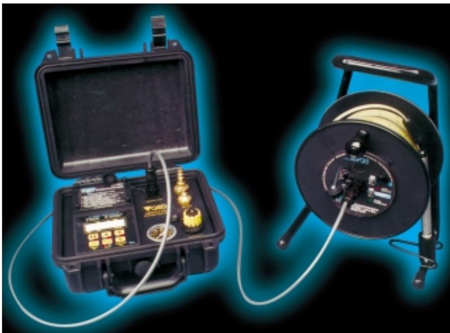
*The MP30 (right) links to the MP10 or MP15 basics Controllers to provide continuous control of well level during low-flow purging and sampling. If the preset maximum drawdown level is reached, the MP30 signals the controller to put pumping on standby mode until the well level recovers.*
