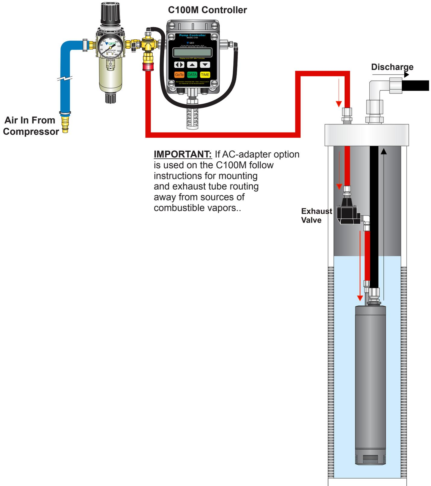
**IMPORTANT:** If AC-adaptor option is used on the C100M follow instructions for mounting and exhaust tube routing away from sources of combustible vapors..
