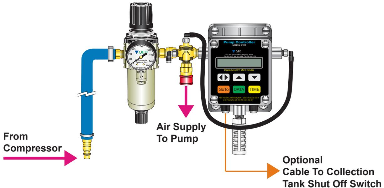
**Model C100M - Powered by external power adapter**, 110V AC input (Not rated for use near explosive or flammable liquids or vapors), VDC output.
