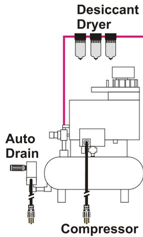
**CAUTION:** Standard compressors not rated for use near explosive or flammable liquids or vapors.
