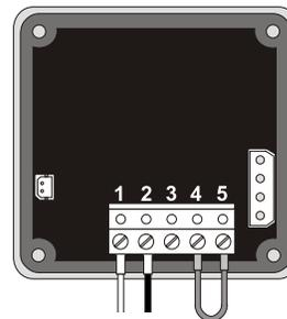
1. Connect leads from level switch to terminals #1 and #2.
