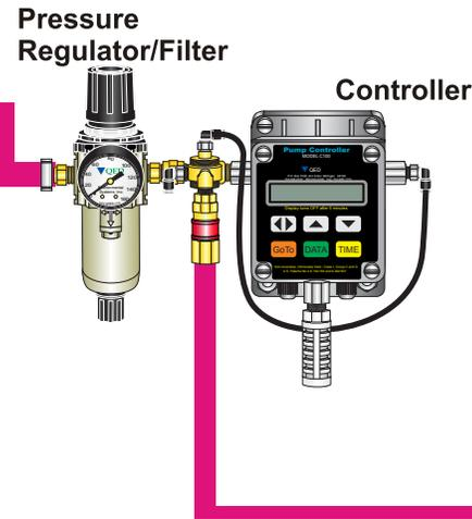
**CAUTION:** The C100M controller in Solar Powered mode is rated for use near explosive or flammable liquids or vapors. All externally powered controllers must be located in a safe area according to local codes
