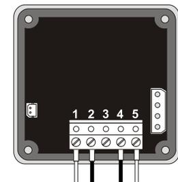
1. Remove jumper wire from terminals #4 and #5.
