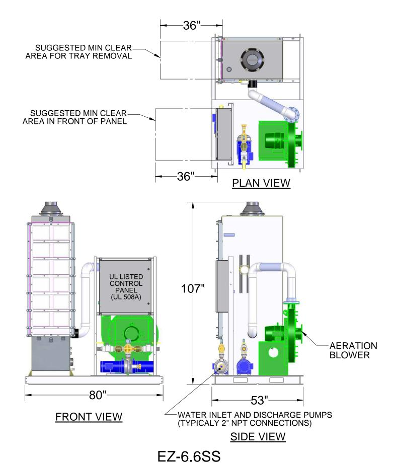
EXAMPLE OF A SKID SYSTEM WITH CONTROL PANEL, PUMPS, AND BLOWER CONTACT QED FOR INFORMATION ON ALL OPTIONS.
