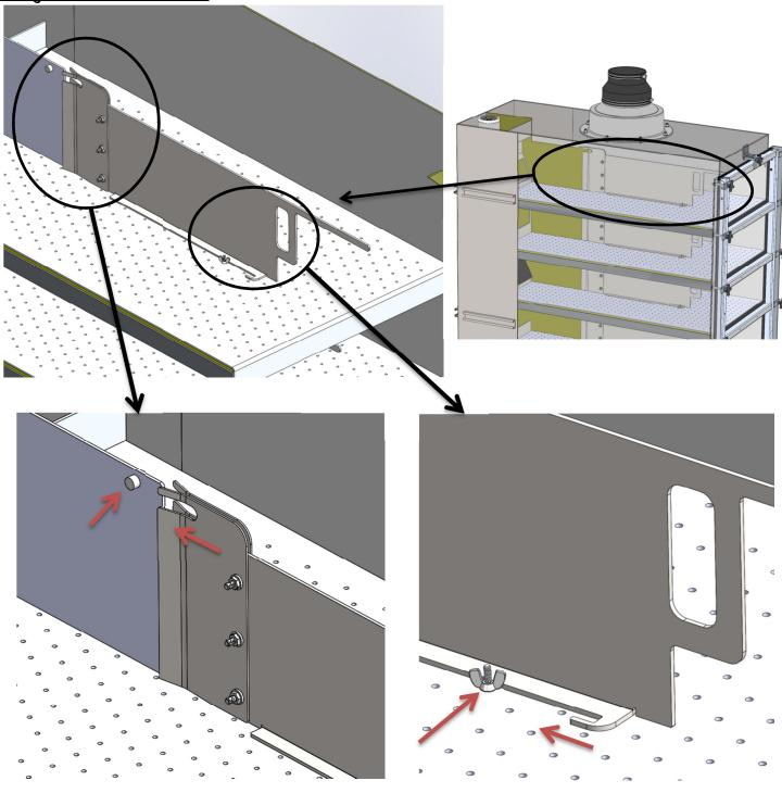
Slide the weir in so that the fixed weir slides in between the two plates and onto the weir pin. Used only on the 6, 8 and 12 series units.
