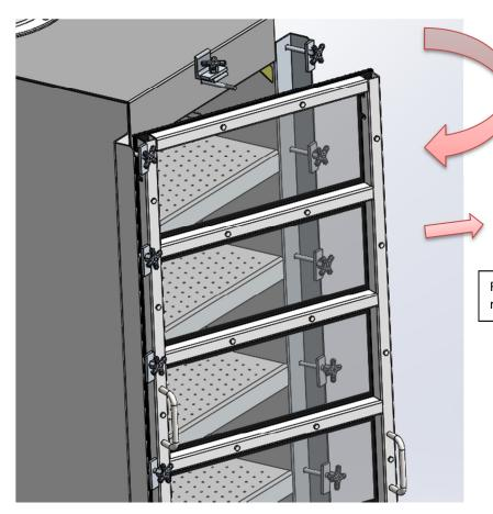
Rotate door and pull out to remove the door
