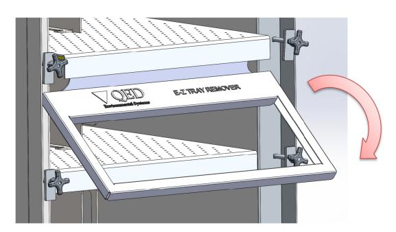
Rotate the tray remover down to loosen the tray. Once the tray is loose the remover is no longer needed
