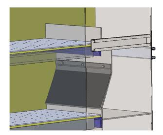
Installed flap (808074) with screws (808039)
