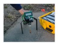
The FROG can also analyze soil samples onsite, detecting volatile organic compounds in soils down to part-perbillion level concentrations.
