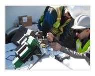
The FROG Portable GC can also be used to monitor your progress at remediation sites with quick, lab-quality results.
