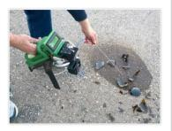
The FROG portable gas chromatograph can detect volatile organic compounds (VOCs) in air, delivering lab-quality results in less than 10 minutes.
