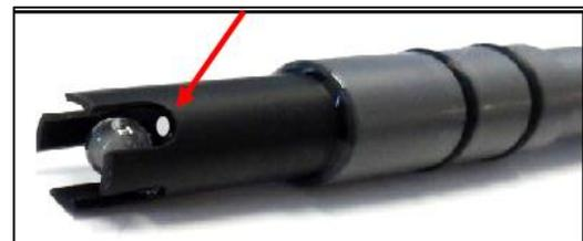
ORP electrode maintenance is also minimal, only occasional cleaning the platinum surface with a soft cloth or soft cotton swab and soapy water. If the platinum is discolored, you can polish the ORP electrode with very light abrasive, like 900-grit wet-and-dry sandpaper or a pencil eraser. You must be careful not to scratch or polish the pH glass bulb.
