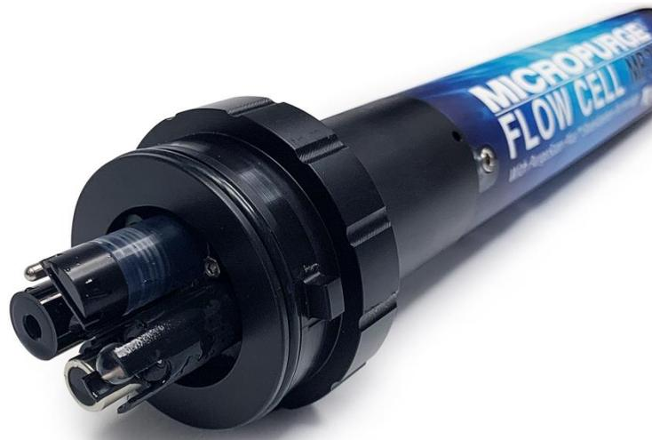
3. Insert sonde/adaptor into flow cell and push into bayonets slots, then turn sonde clockwise to lock.
