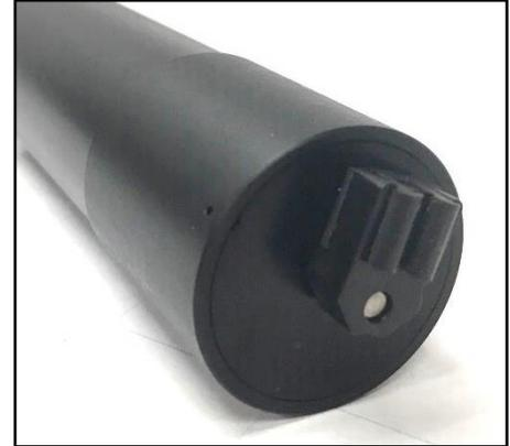
Turbidity sensors require no regular maintenance, but you should check occasionally to make sure the optical window has not been scratched or damaged by cleaning or accidental contact.
