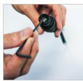
Using a 3mm allen wrench, release the nut inside the filter holder
