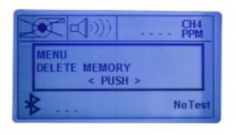
NOTE: The SEM5000 will store up to 480 hours of scan data before the memory must be deleted.
