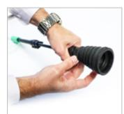
Unscrew and remove windscreen from the end of the sample probe
