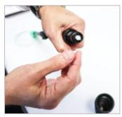
Once the windscreen has been removed, remove and discard the cellulose filter from the filter holder at the end of the wand
