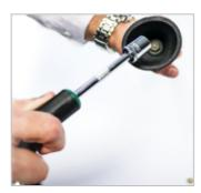
Using a 13mm socket, unscrew the bronze dust filter and remove it from its position inside the windscreen
