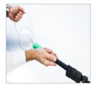
Remove the old tubing from the handle end of the sample probe
