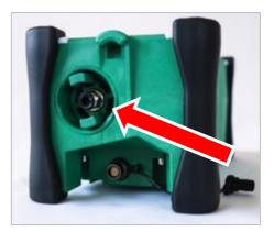
NOTE: If the tube is not fully inserted into the sample inlet of the SEM5000, the concentration readings during field calibration may appear to be erratic and difficult to stabilize.
