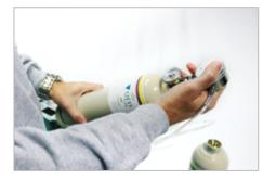
NOTE: The regulator flow must be a minimum of 0.6L/min to avoid restricting the pump. The SEM5000 package is provided with one demand-flow regulator with a C10 fitting. It is recommended that two regulators be used, (one per bottle), for ease of calibration.
