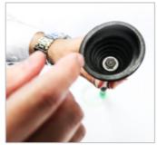
Tighten the filter with your fingers and, if necessary, use the 13mm socket for final tighten
