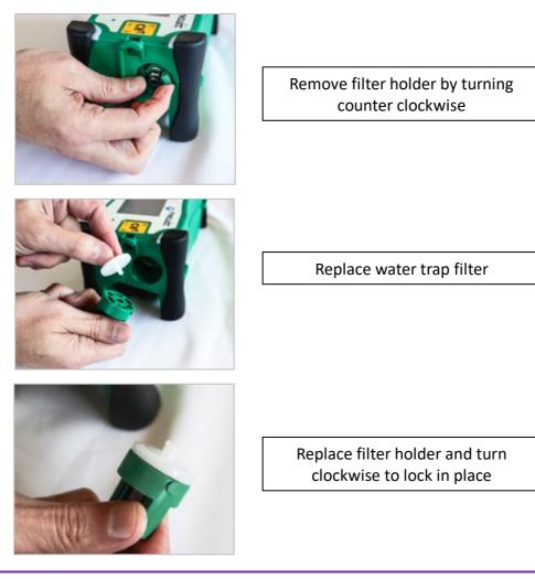
NOTE: The water trap filter should be checked and changed periodically. It is recommended that it be changed prior to each SEM event. At a minimum, it should be checked quarterly and is recommended to be checked weekly during periods of heavy use.
