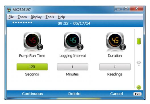
5. Press key 2 to enter **Logging Interval**, then enter 3 minutes and press Enter when complete
