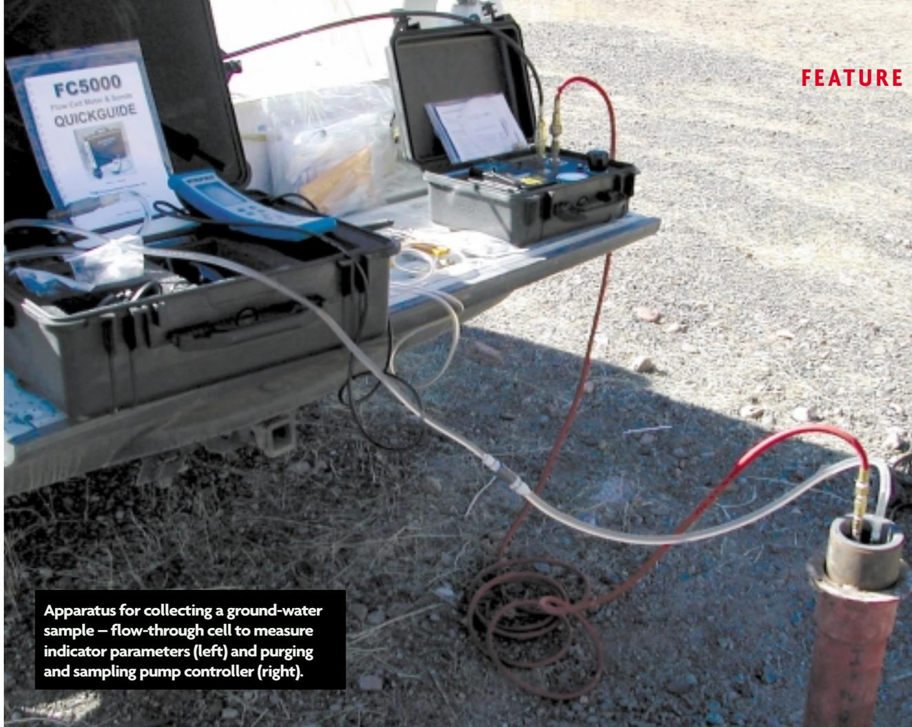
Apparatus for collecting a ground-water sample — flow-through cell to measure indicator parameters (left) and purging and sampling pump controller (right).
