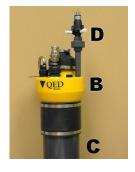
4. Install the QED LFG wellhead assembly (E) into the well cap (B)(refer to LFG well cap installation instructions).
