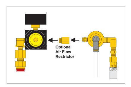
**NOTE:** An optional air flow restrictor is included with the L600 to restrict the air flow through the pump, if necessary, in wells where pump rates are less than 1/2 G.P.M. or where the pump is submerged less than half the pump length.
