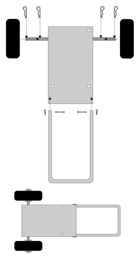
Assemble handle and wheels to cart frame as shown, using cotter clips provided.
