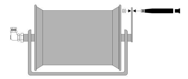
Install reel handle to reel crank arm, using nut and washer provided. Insert plug into end of handle and tighten with allen wrench.
