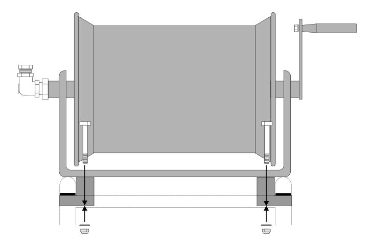
Position frame clamps under reel to grip MP40 frame tube as shown and tighten bolts and nuts securely
