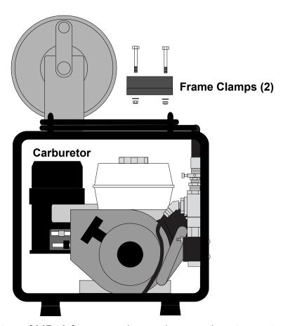
Position Hose Reel on top of MP40 frame as shown, (over carburetor, not over gas tank). Use care to avoid having the reel fall off the frame.
