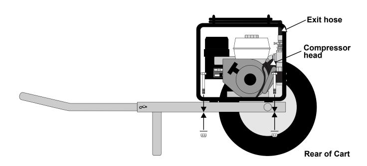
Mount MP40 to frame by removing 4 rubber feet, then bolting the MP40 to the frame with the bolts provided.
