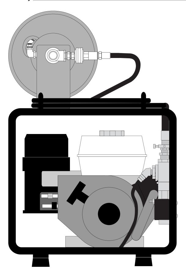
Attach the quick connect fitting from the compressor hose to the quick connect fitting at the center of the hose reel .
