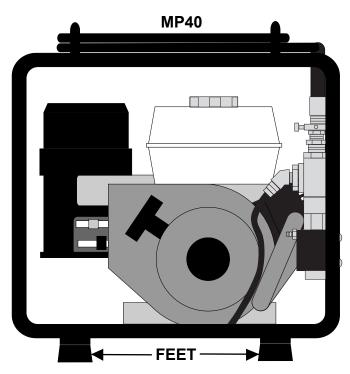
Remove rubber feet (4) from bottom of MP40 Frame.
