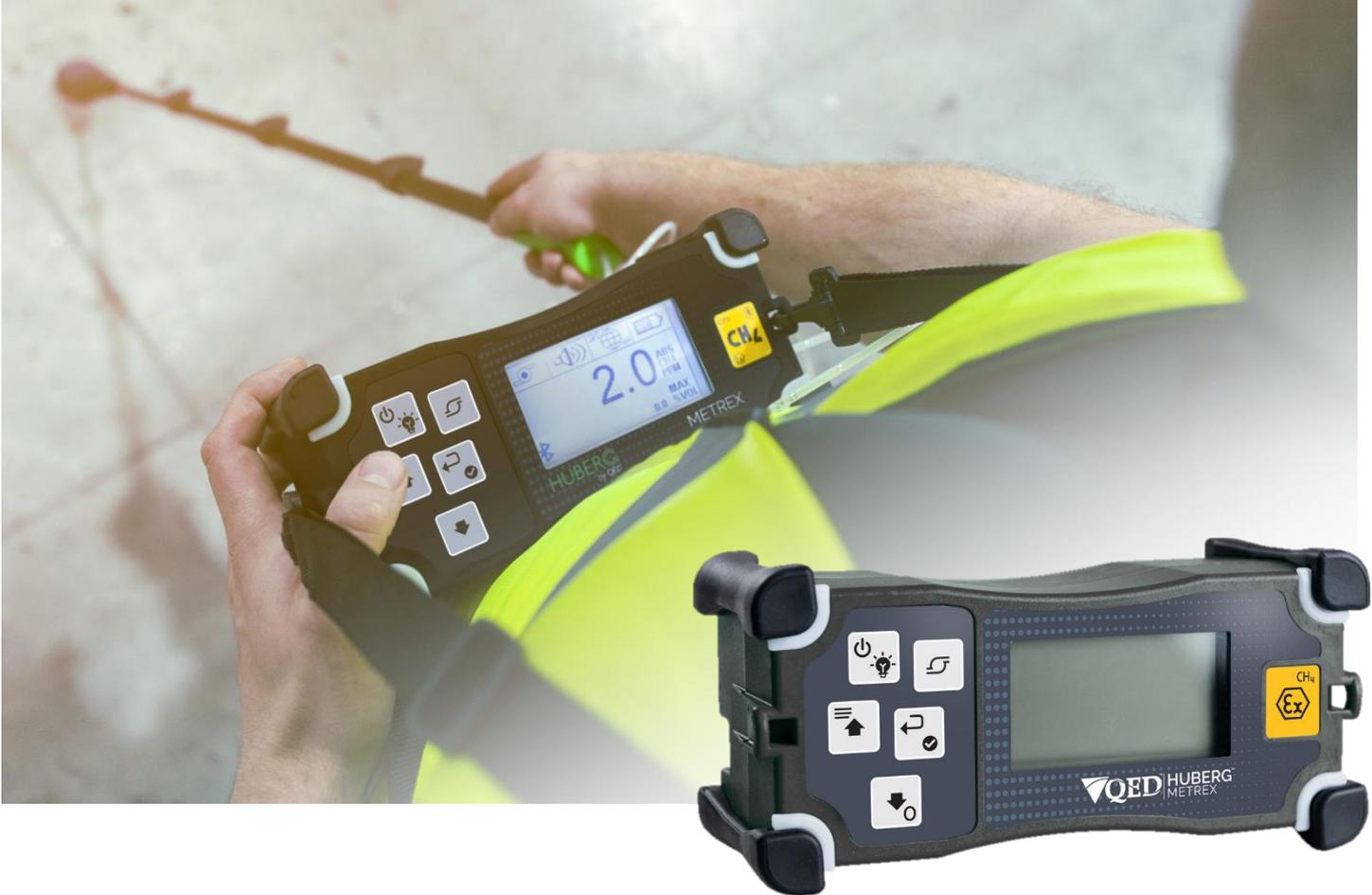
The METREX instrument is ATEX certified and designed for pre-localisation, localisation and classification of natural gas leaks in gas distribution networks
