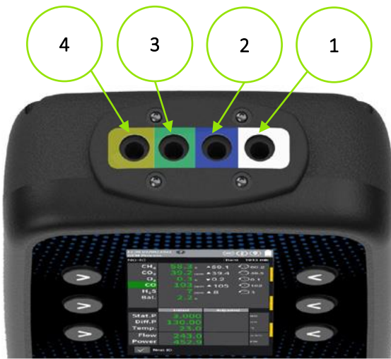
Figure 3 – Pro Series Connections
