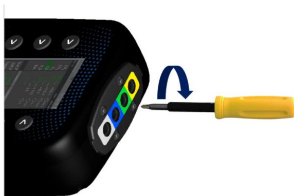
Figure 15 – Inlet Port Plate Fitting
