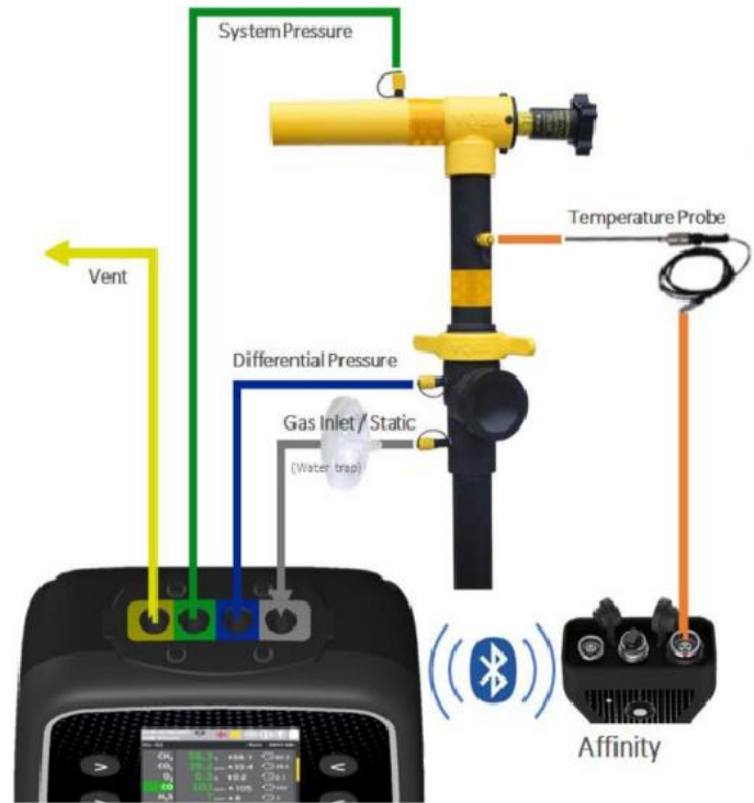
Figure 4 – Pro Series Connection to QED Wellhead
