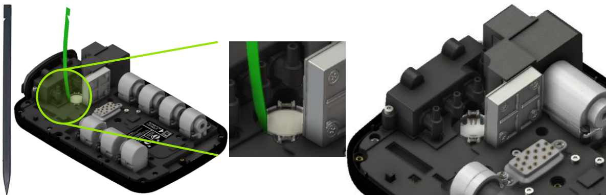
Figure 11 – Coin Cell Removed
