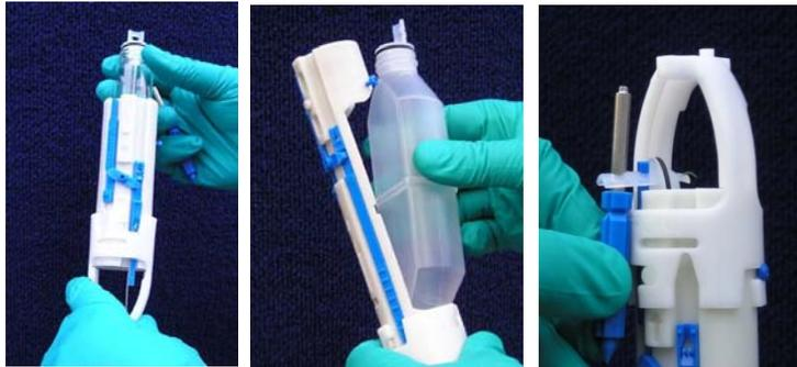
The equilibration period for the Snap Sampler depends on the installation environment and the analytes of concern. For many inorganic analytes, Snap Samplers have been shown by the US Army Corps of Engineers to be in an equilibrium state within the shortest timeframe measured in their tests—24 hours. For organic analytes, including
